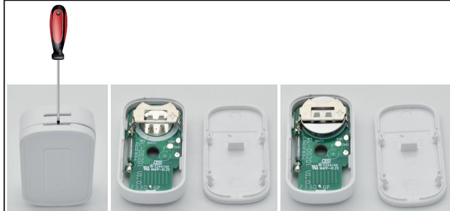
If the LED does not light up when the magnet is removed, replace the battery 1632.
