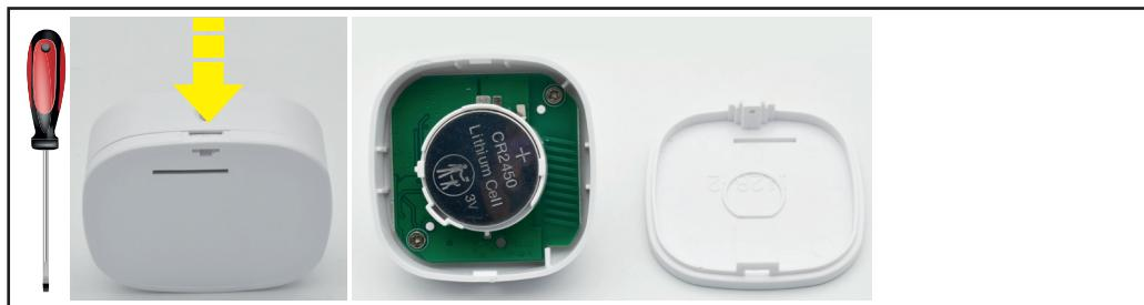
If the LED does not light up when passing in front of the sensor, replace the battery 2450.
