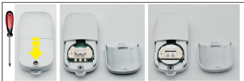
If the LED does not light up when a button is pressed and/or the remote control does not function, replace the battery 2032.
